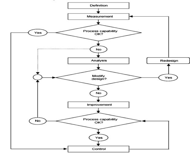
The flowchart for DMAIC: The Six-sigma Methodology is sketched in figure below:
