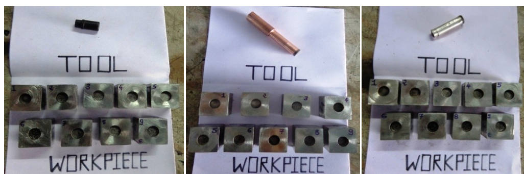
Fig 3. Tool & Workpiece Material after Machining : Graphite, Copper, Silver
